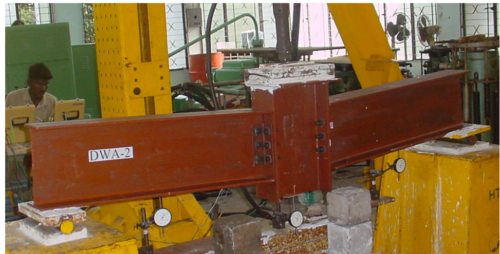
a Deformed shape of the connection
