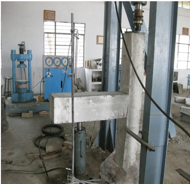
Fig. 7 Experimental test set-up of exterior beam-column joint
