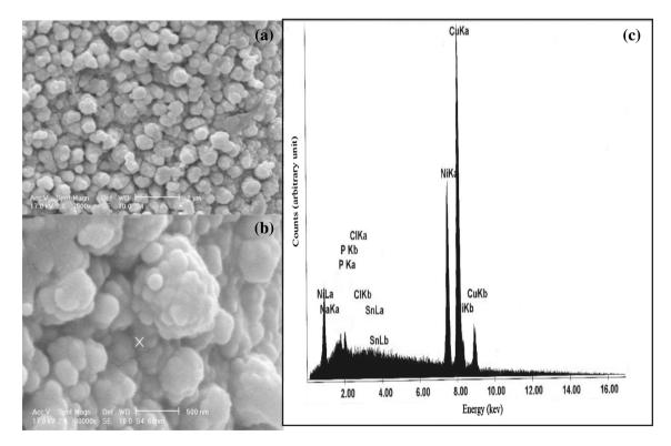
Fig. 9 SEM image of Cu-Ni-P-Ni electroless plated PET fabric a ×7500, b ×80,000, c the EDAX analysis of Cu-Ni-P-Ni-coated layer
