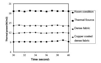
Fig. 4 Recorded thermal radiation by thermopile sensor for different condition
