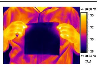
Fig. 12 Captured thermal image from human body while keeping a piece of dense Cu–Ni–P–Ni composite nanoparticle-coated fabric
