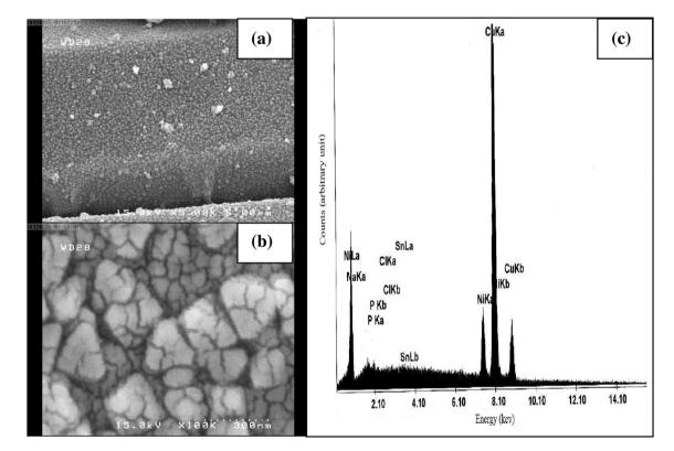
Fig. 3 SEM image of copper electroless plated a 5000×, b 10,000×, c the EDAX analysis of Cu-Ni-P-coated layer
