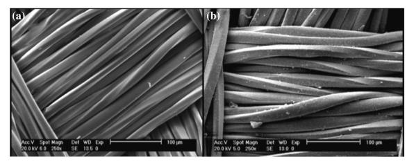
Fig. 2 SEM image of a the neat PET fabric, b Cu-Ni-P electroless plated
