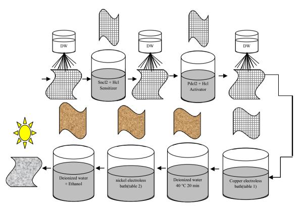
Fig. 1 Graphical representation of Cu-Ni-P-Ni plating procedure
