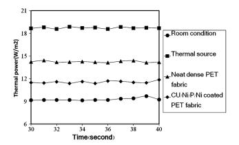
Fig. 10 Recorded thermal radiation by thermopile sensor for different condition
