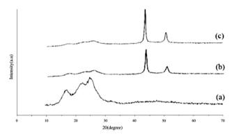
**Fig. 13** XRD spectra of metallic fabrics: **a** untreated PET fabric, **b** Cu–Ni–P fabric I (1 1 1) = 13.13, I (2 0 0) = 4.75, **c** Cu–Ni–P–Ni fabric I (1 1 1) = 17.16, I (2 0 0) = 6.33
