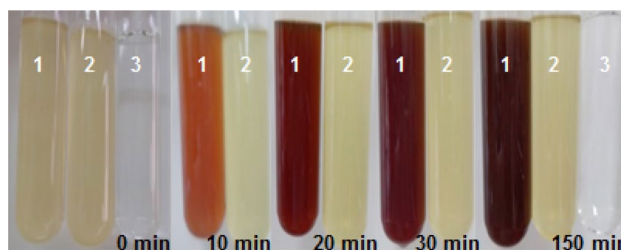
Fig. 1 Monitoring of the color changes in the reaction medium of the AgNP synthesis produced with aqueous extracts of P. emarginatus leaves collected during the summer. In this representation, 1 refers to AgNPs synthesized with P. emarginatus leaf extract at 10%; 2 refers to a control composed of only aqueous extract at 10%; and 3 to a control with only the silver nitrate solution at the final concentration of 1 mM
