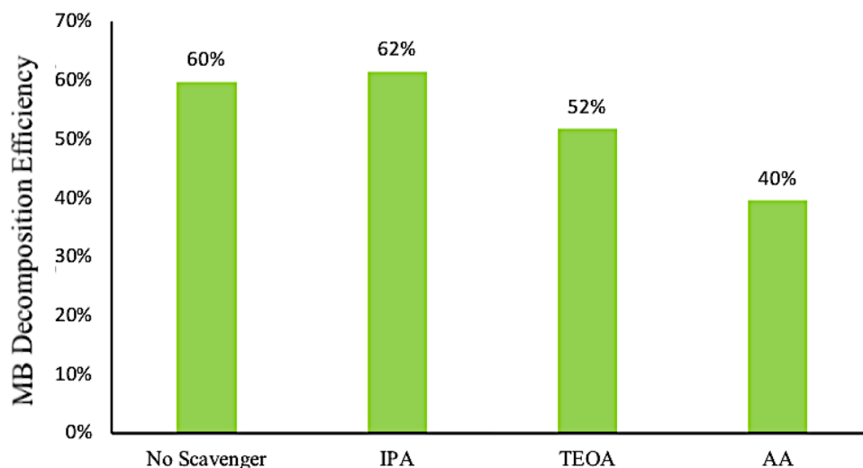
Fig. 9 The active species trapping experiments for TCF photocatalyst sample via different scavengers (initial dye concentration: 10 ppm; volume: 100 mL; catalyst dosage: varying between 5 and 30 mg, illumination time: 240 min)
