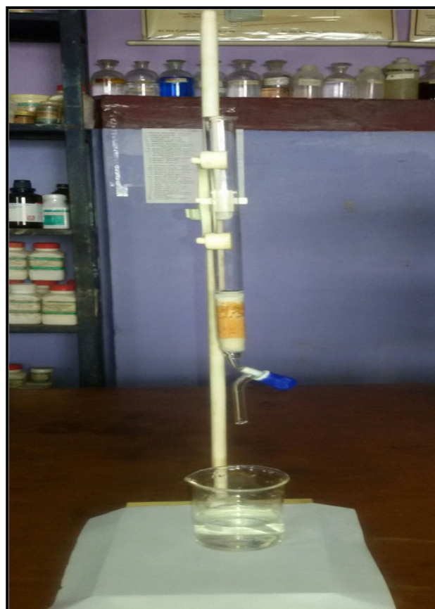
Fig. 2 Column used for the removal of pollutants from composite
