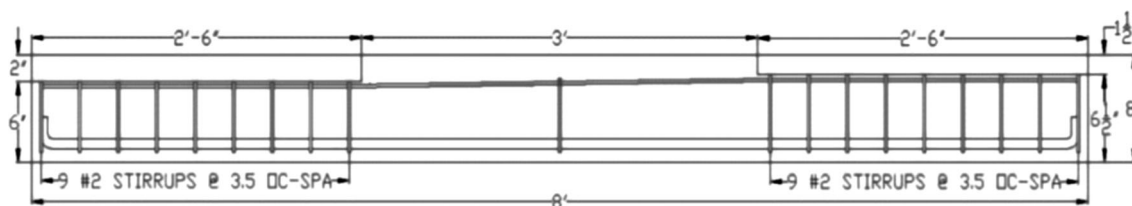
Fig. 7 Full-scale beam elevation dimensions.
