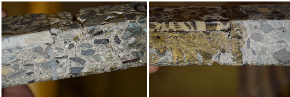
Fig. 13 Prototype failures; inorganic (left), organic (right).
