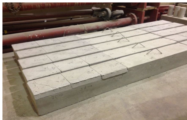
Fig. 9 Notched full-scale beams.
