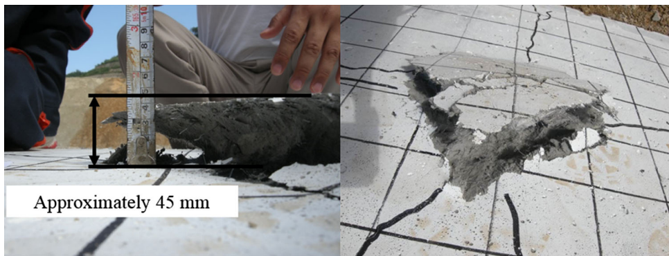
Fig. 13 Fragment of the back side of the PVASCC panel in case of blast charge of 200 g.
