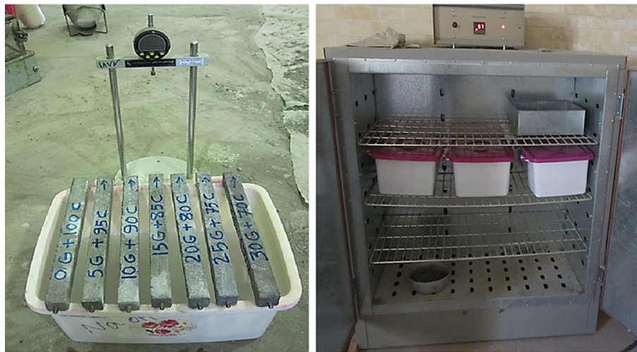
Fig. 19 Mortar bars stored in a 1 N NaOH solution at 80 °C.
