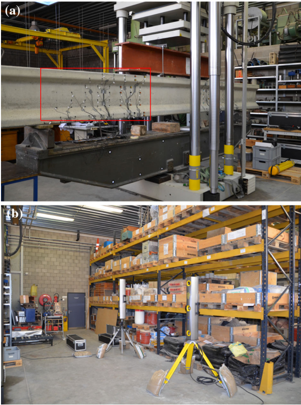
Fig. 3 Experimental setup for the adopted coordinate measurement machine (CMM): a IR LEDs (indicated with red rectangle); b Camera units mounted on tripod.
