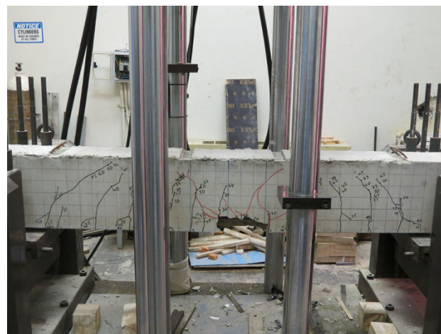
Fig. 11 Cracked bond beam (SCC-B-B2).
