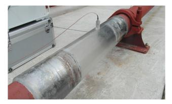
Fig. 5 Application point of the UVP and transparent engineered plastic.
