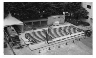
Fig. 4 Overview of the 170 m full-scale pumping setup.
