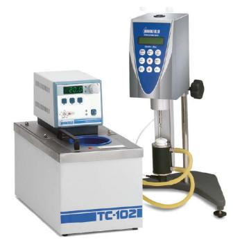
Fig. 3 Rheometer for the measurement of rheological properties of mortar and cement paste.
