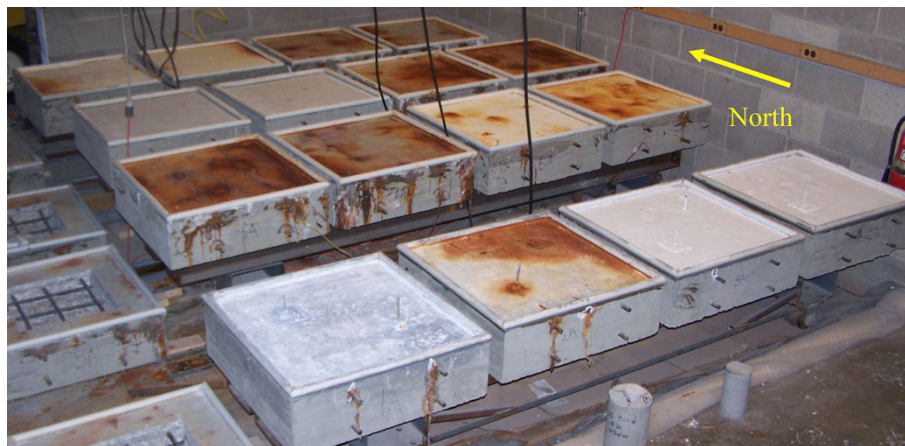
Fig. 12 Surface staining on laboratory specimens after 6 months.
