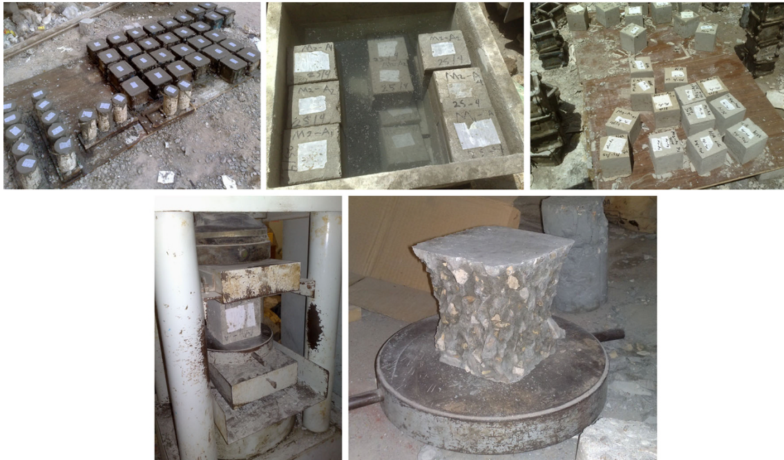
Fig. 4 Concrete cubes preparation, curing, and under compression testing.
