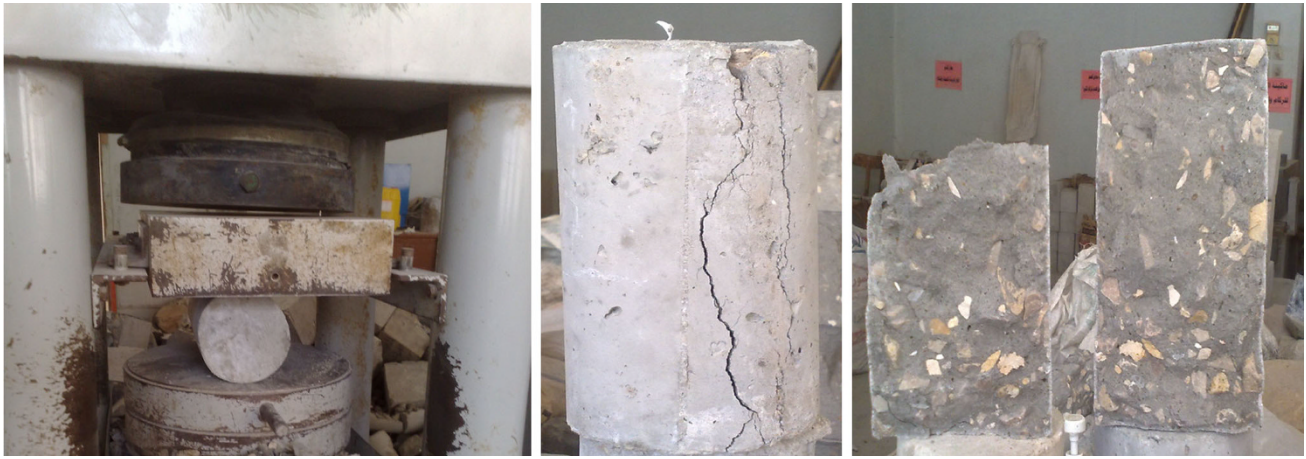
Fig. 7 Split tensile strength test.
