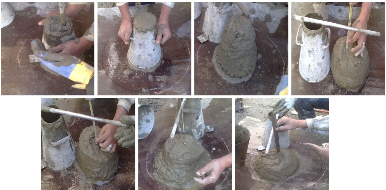
Fig. 3 Slump for mixtures with different cement replacement.
