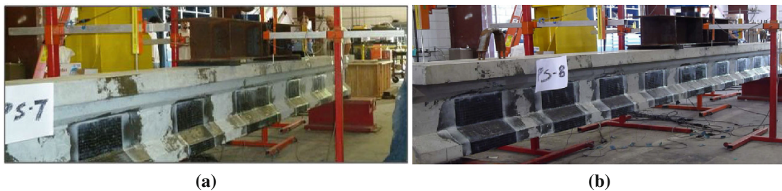
Fig. 8 Girder test setup diagram and photo of specimen during testing. a Static testing of PS-7. b Static testing of PS-8.
