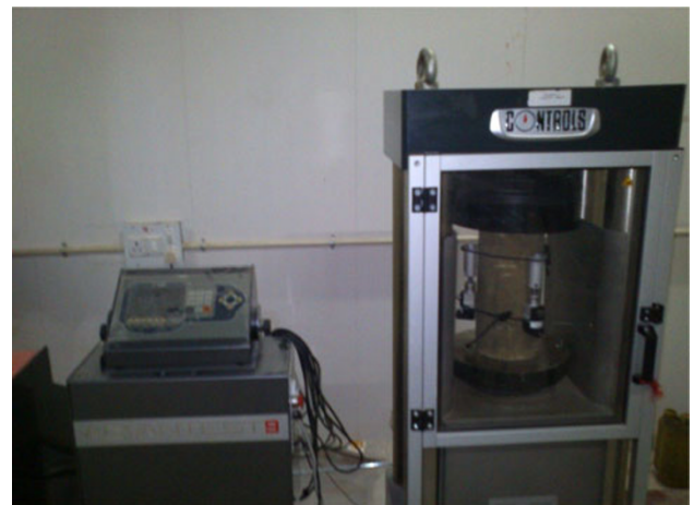
Fig. 2 Test set up for determining the elastic modulus.
