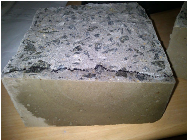
Fig. 4 Water penetration depth front marked after the test.
