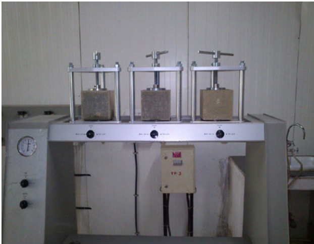
Fig. 3 Permeability test set up for determining the water penetration depth.
