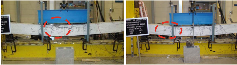
(a) Flexural Failure
