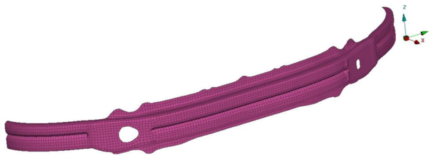
Fig. 25 Bumper geometry modified during iteration 3(IO03) (length = 1586 mm, thickness = 2 mm)
