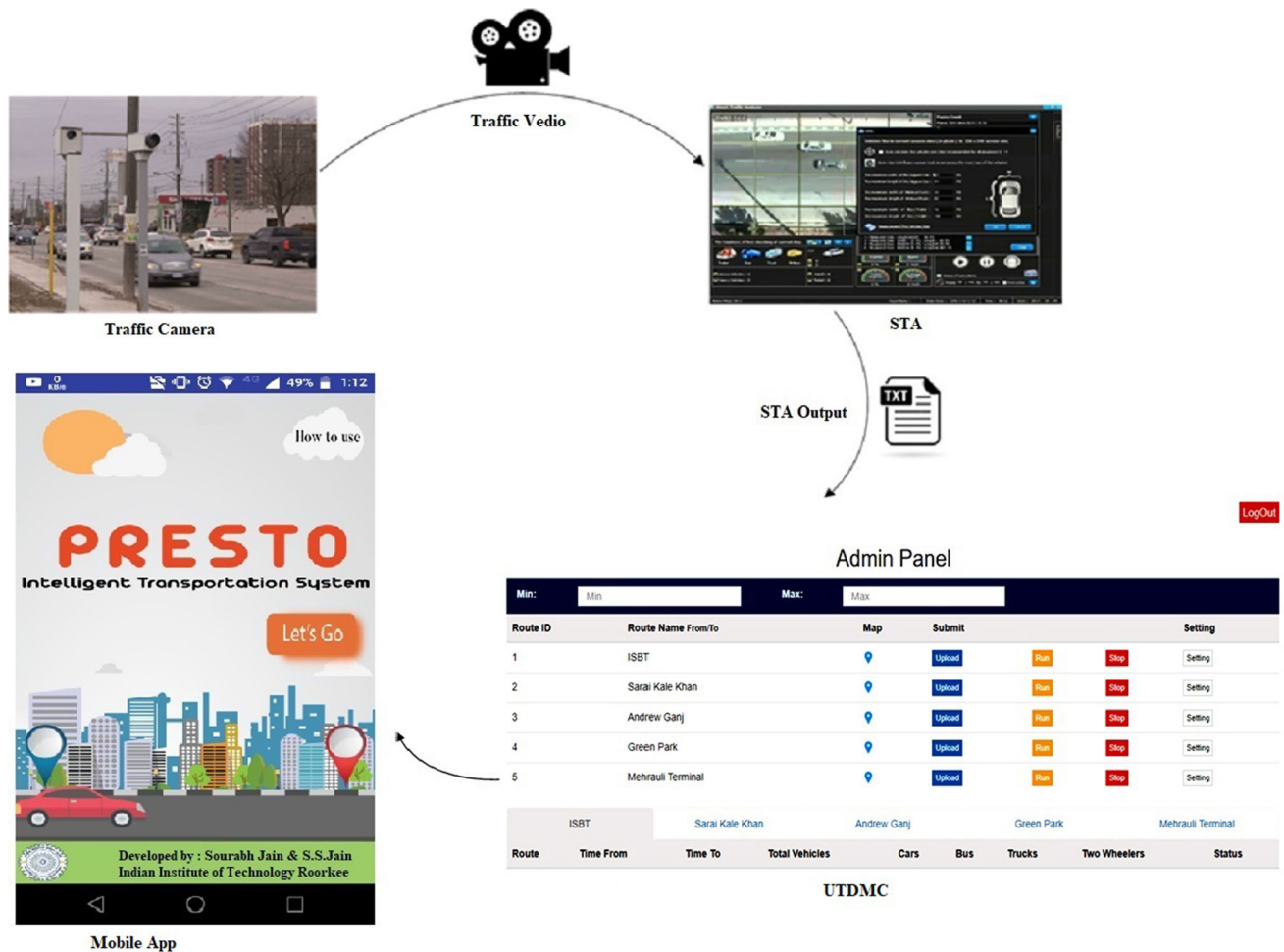
Fig. 1 Intelligent transportation system flow diagram
