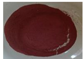
(c) Calcined sludge ash
