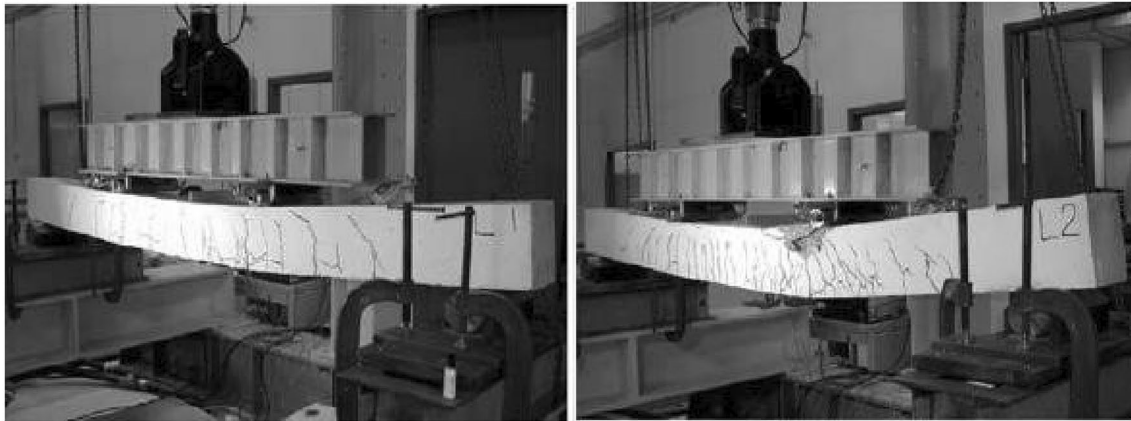
Fig. 9 Cracks patterns for hybrid-reinforced beam [63]
