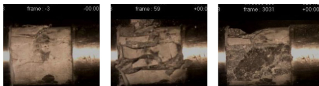
Fig. 13 High-speed photography of specimen failure process in the case of P_{as} = 24 MPa and \dot{\epsilon} = 99.66 s ^{-1}
