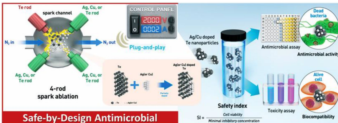
Fig. 3 Schematic of spark ablation used to prepare Ag or Cu-doped Te nanoparticles from three Ag or Cu anodes (green) and a Te cathode (red) inside a chamber under a nitrogen gas flow. The given figure was adopted from Park et al. (2019)
