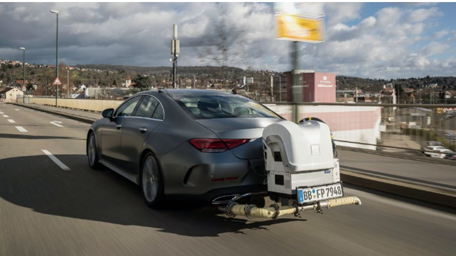
Portable emissions measurement systems are used to test vehicle emissions in real driving conditions
