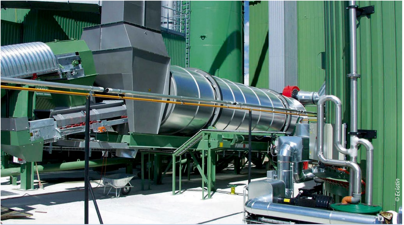
In Langenthal in Switzerland, the Ammann Group manufactures asphalt mixing machines, which are coated with polyaspartic systems. The paint is supplied by Eclatin AG, a company also based in Switzerland.
