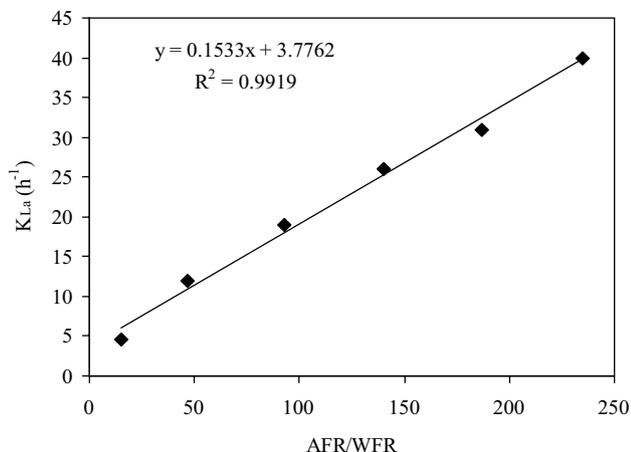
**Fig. 5** Relationship between oxygen mass transfer coefficient and AFR/WFR for MS-FFBR
