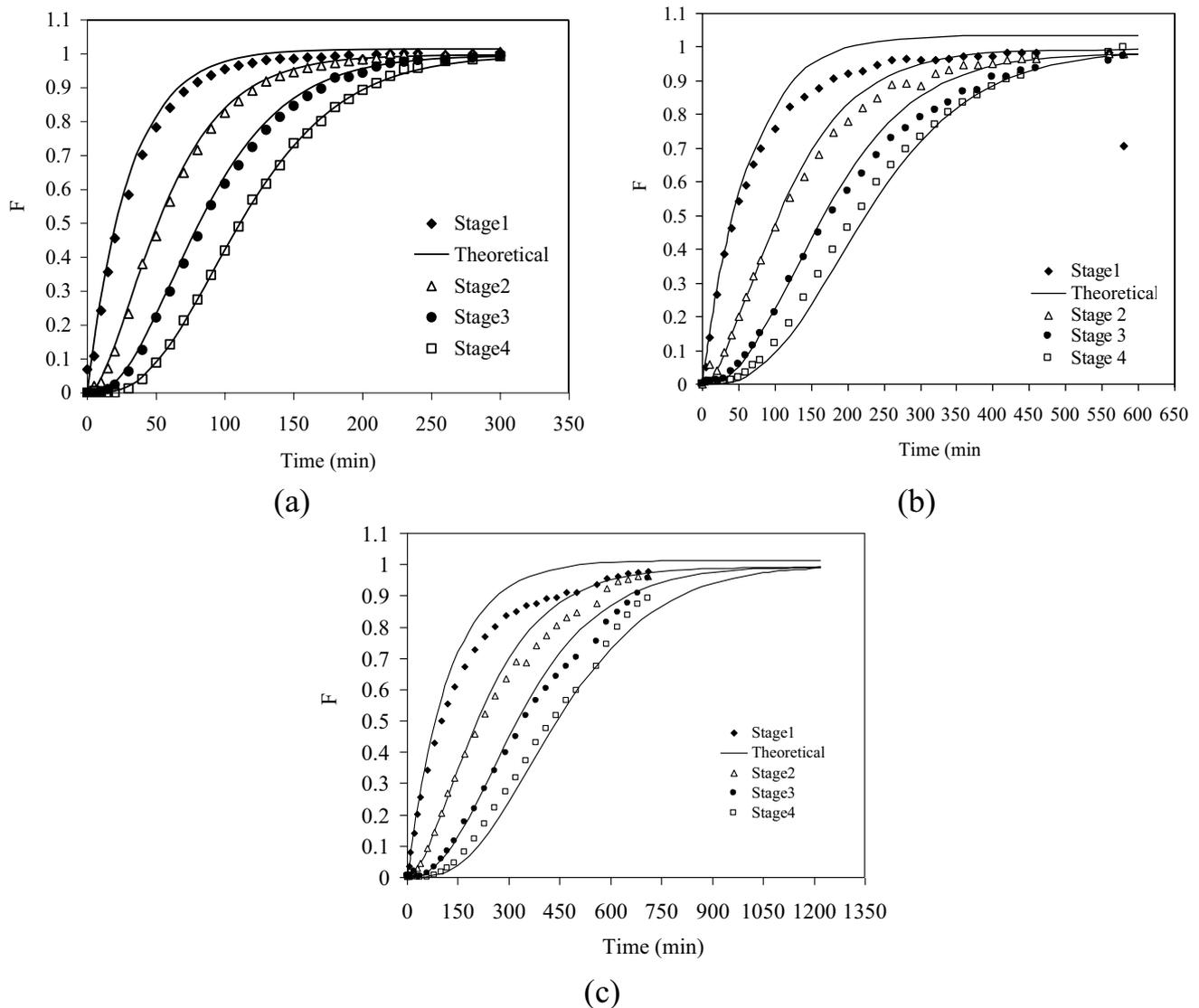
**Fig. 3** Residence time distribution of F-curve for four compartments in series at various HRTs of **a** 2 h; **b** 4 h; and **c** 8 h
