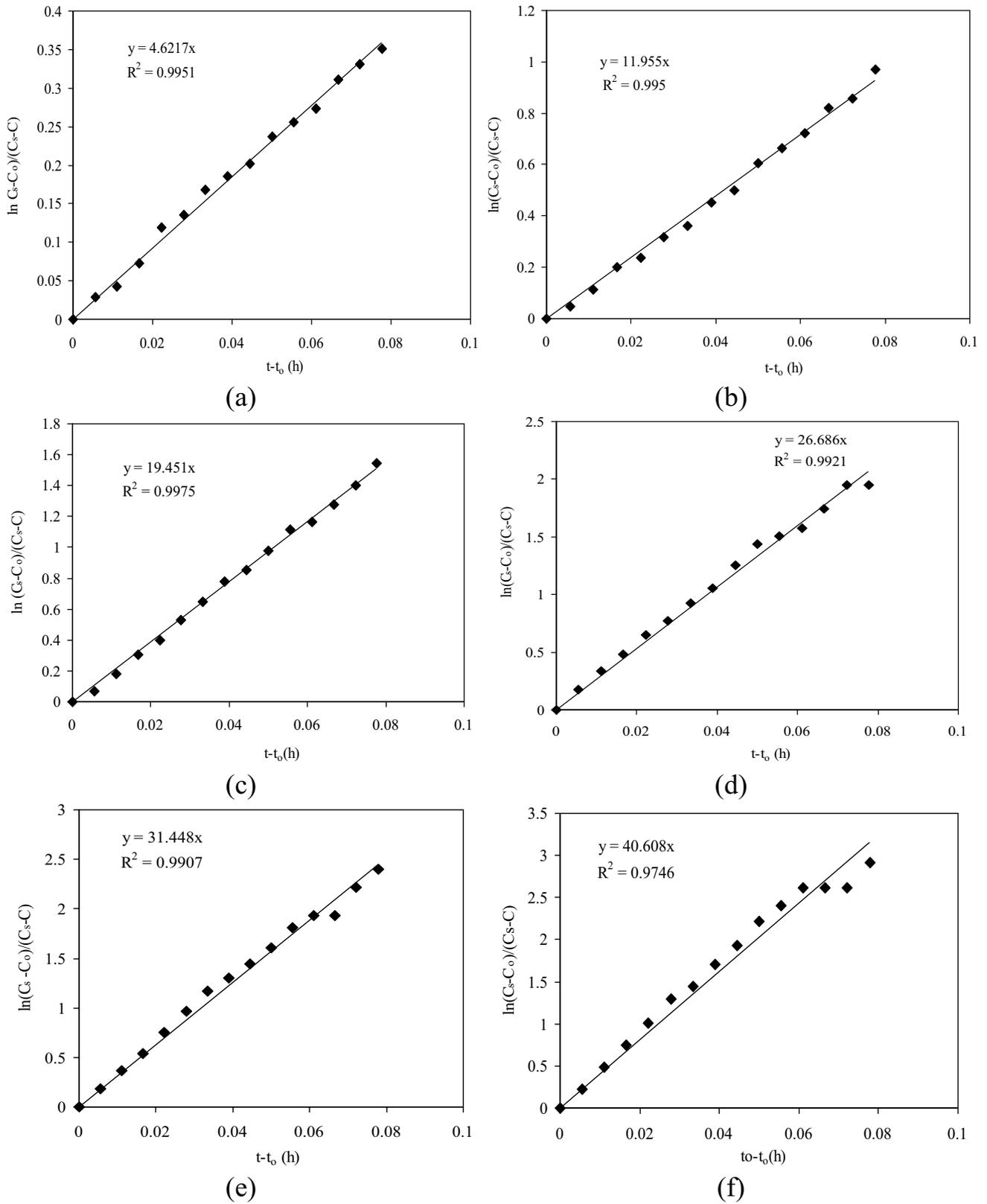
**Fig. 4** Regression plots used for determination of oxygen mass transfer coefficient at various AFR/WFR of **a** 14.4; **b** 47.5 **c** 93; **d** 140; **e** 187; and **f** 235
