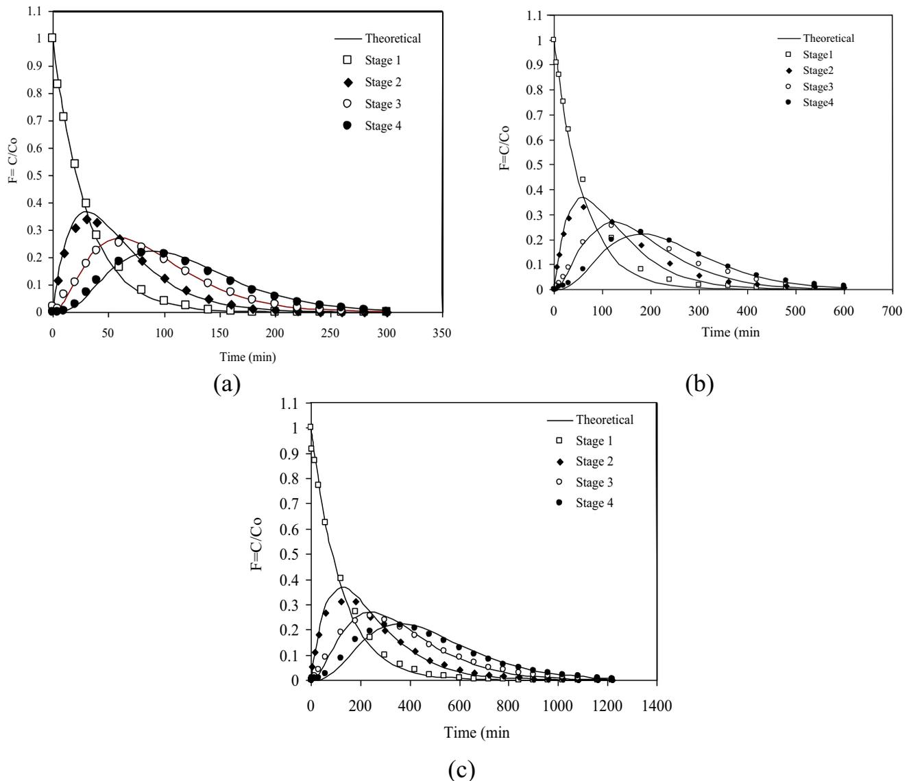
**Fig. 2** Residence time distribution of C-curve for four compartments in series at various HRTs of **a** 2 h; **b** 4 h; and **c** 8 h
