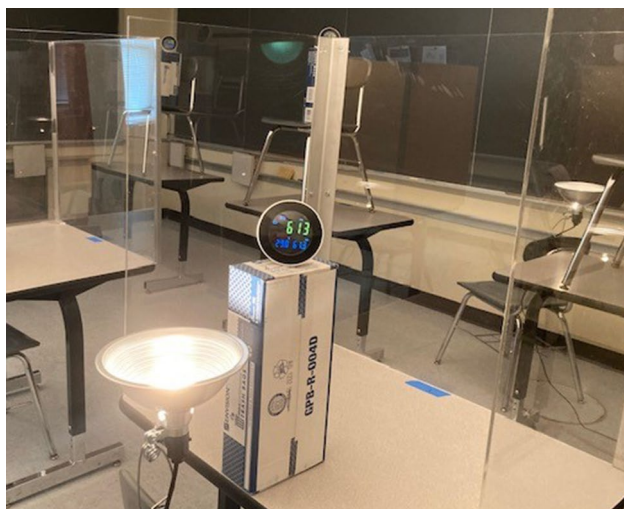
Fig. 3 Desk dividers. A sample test setup. In the foreground is Desk 7 (pictured XT-10 CO 2 monitor) with its associated heat lamp. Visible in the background are instructor stations 9–11. Only one lamp was used for the instructor and was placed in the middle of the instructor row
