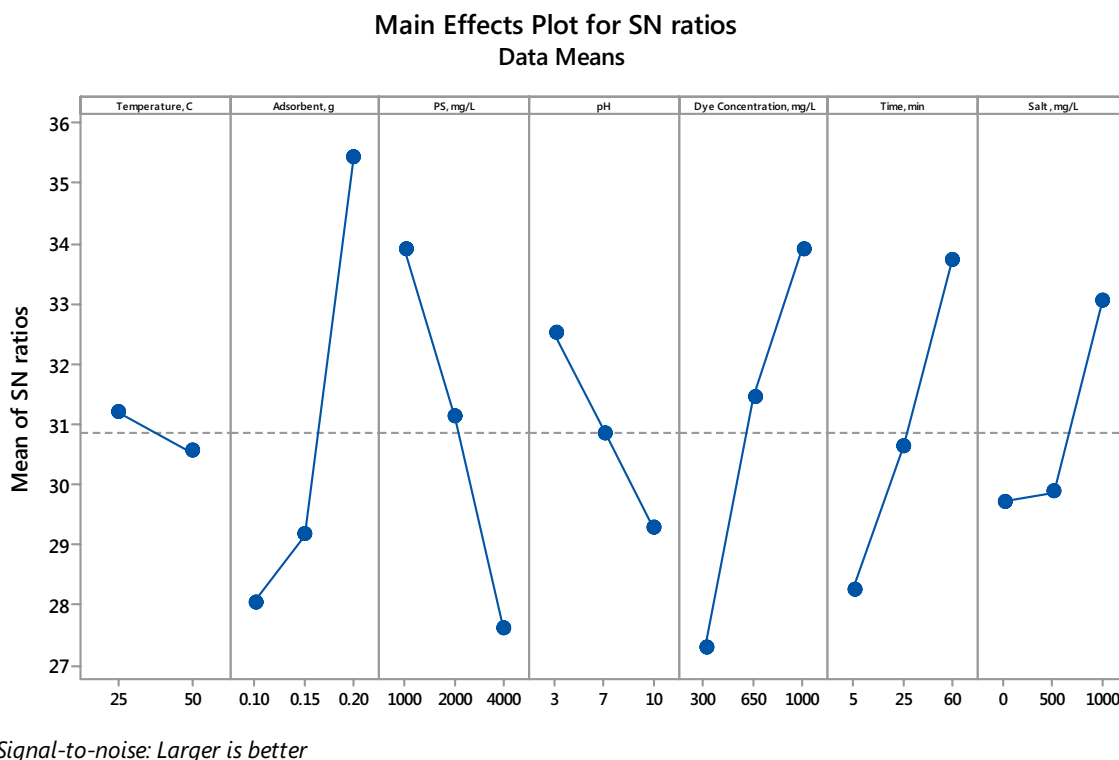
Fig. 5 S/N ratios of operating parameters on COD removal for HPS
