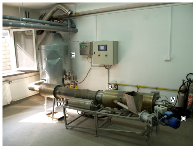
Fig. 1 High scale rotary kiln
