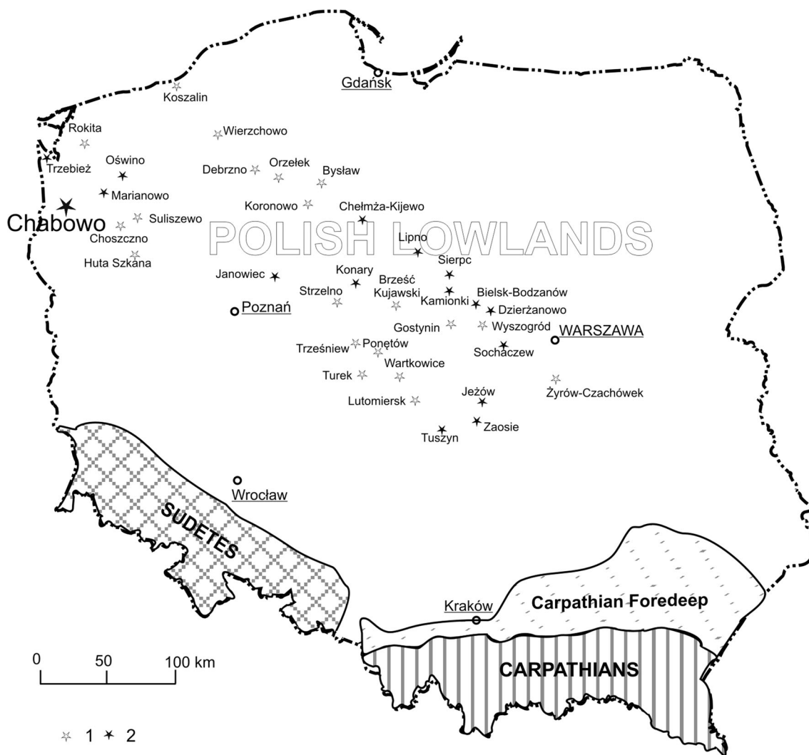
Fig. 1 Potential geological CO 2 storage sites in the Polish Lowlands. Explanations: 1 structures with one level of CO 2 storage, 2 structures with two levels of CO 2 storage
