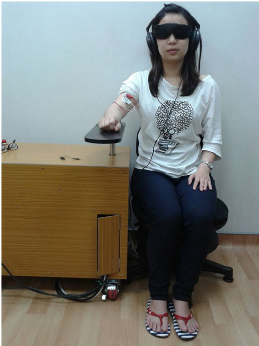
Fig. 1 Proprioceptive apparatus experimental setup. Participants sat on a chair with their vision and hearing occluded. Each participant's forearm was placed on the splint, with the elbow at 90°. EMG electrodes were positioned over the biceps brachii to monitor muscle activity during the trials
