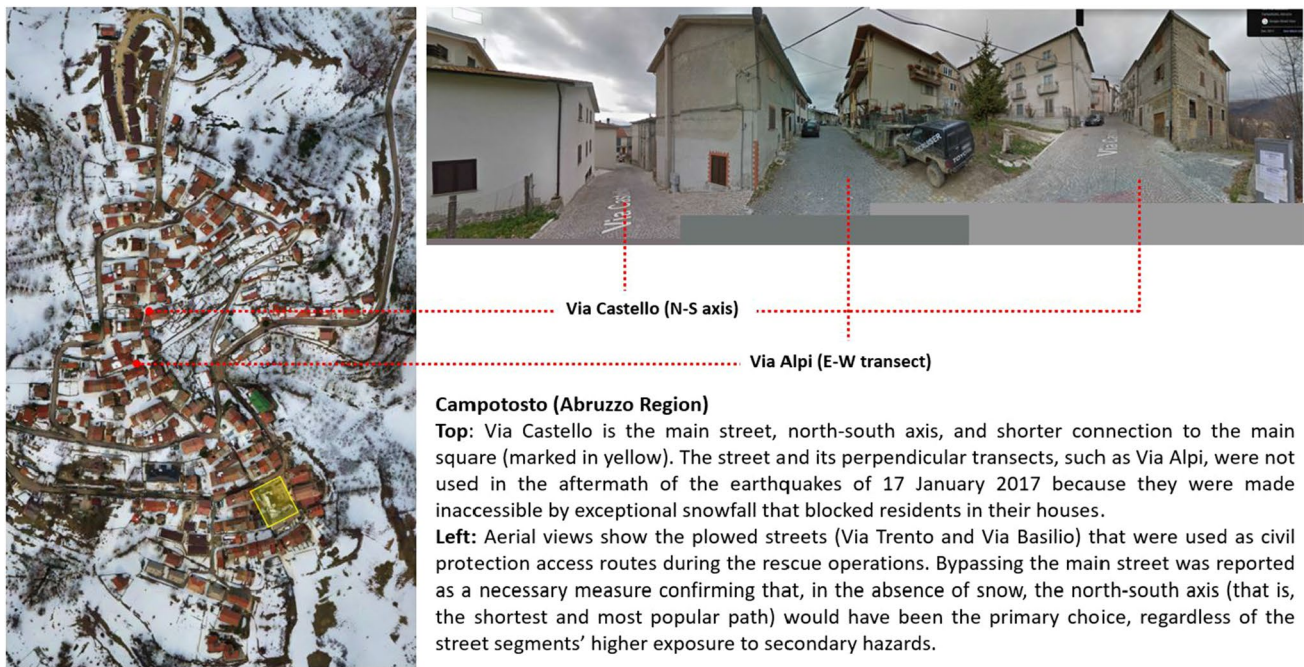
Fig. 3 Aerial view and street view composition of Campotosto, case study from the Abruzzo Region and epicenter of the 17 January 2017 earthquake. Image sources Author elaboration on Google Street View; aerial view courtesy of Norcia Fire Brigades
