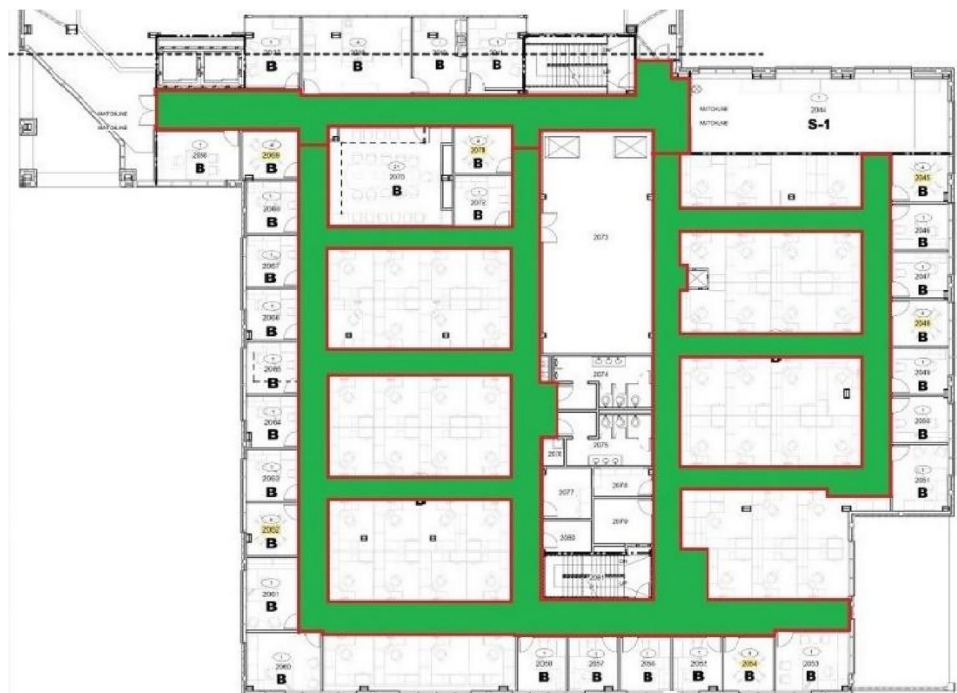
Fig. 1 Workplace floor plan, with desired coverage area for the 2D problem depicted in green color. For the 3D problem, the interior of cubicles (large rectangular rooms outlined by the corridors in green color) is subject to coverage as well.
