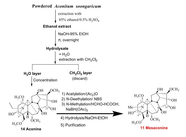
Fig. 4 Industrial preparation process for Mesaconine (11)
