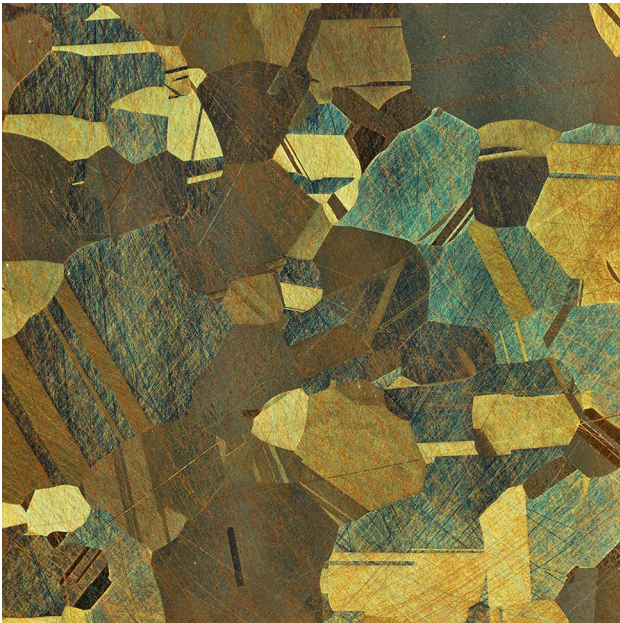
Fig. 6 Klemm's III applied for 4 min image with polarized light
