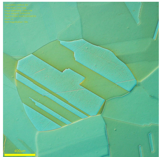
Fig. 9 Klemm's III applied for 8 min after polishing to 0.05 \mu\text{m} finish
