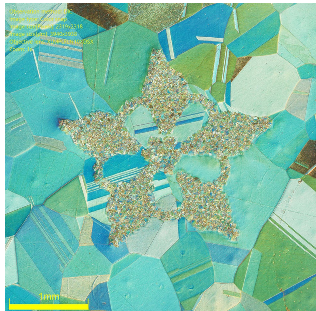
Fig. 12 Columbine flower with shaded petals imaged with polarized light
