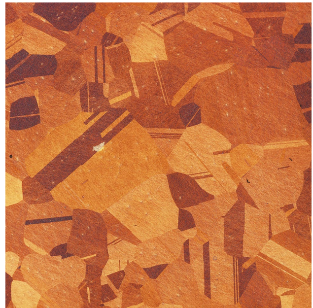
Fig. 4 Klemm’s I applied for 90 s imaged with polarized light
