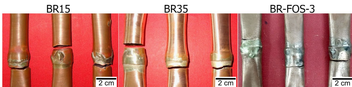
Fig. 8 Specimens for uniaxial tensile testing after fracture using the BR15, BR35 and BR-FOS-3 filler metals
