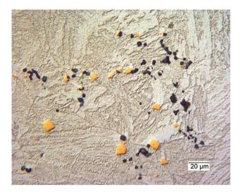
The matrix is steel, but can you name the black and gold second phases? The second phases in the steel matrix are yellow cubic TiN particles and purple/black particles of alumina mixed with MnS.
