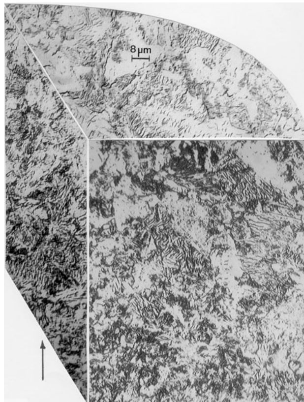
Fig. 10 3D-LOM composite view for dual-phase \gamma -TiAl microstructure representative of the EBM-fabricated cylindrical solid (Fig. 2). The build direction is indicated by the arrow (left)
