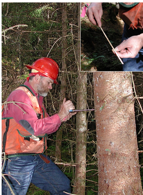
Fig. 1 Increment borer being used to extract a core sample from a tree at breast height (photo credit: Xiping Wang)
