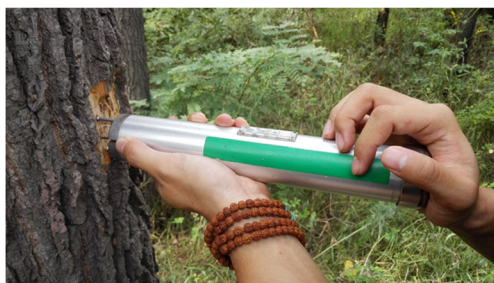
Fig. 3 The Pilodyn Wood Tester measuring the depth of needle penetration into the wood (photo credit: Shan Gao)
