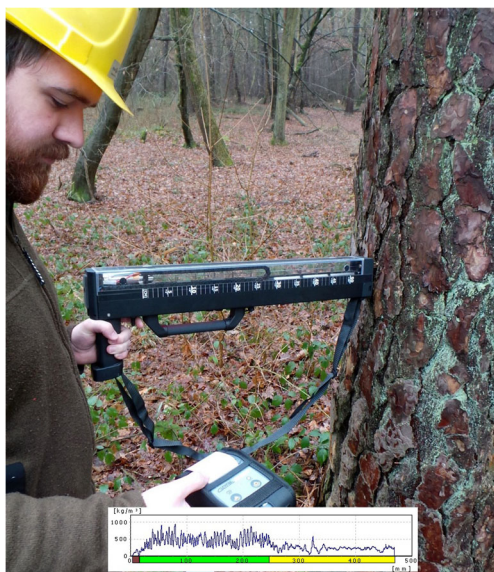
Fig. 5 Electronically regulated resistance drilling in a standing tree using a Resistograph® tool (photo credit: Frank Rinn)
