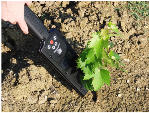
Fig. 4 Microchips were read electronically by 14-length identification number, and the reading can be performed by mobile devices. According to plant growth rate, readers have to guarantee a sufficient reading range in order to retrieve data after years from tagging. Note that the reader is positioned a few centimeters from the grapevine trunk in proximity to microchip location
