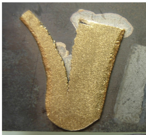
Fig. 3 Crack deformation sample (70 %) of Au-Ge micro alloy
