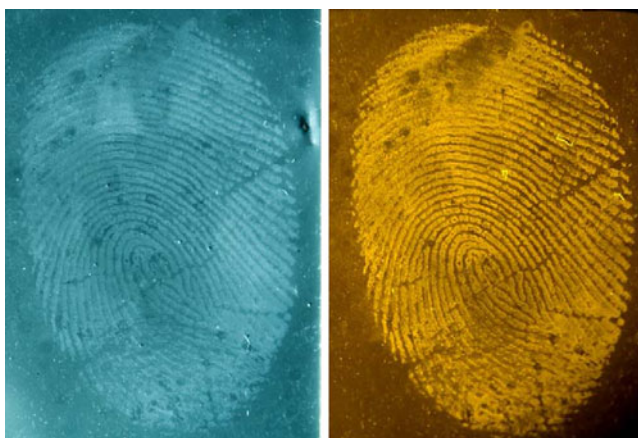
Fig. 3 Latent fingerprint deposited on a black polyethylene bag after the deposition of ZnO. The left picture was observed under a blue light. The right picture was observed under a 300–400-nm luminescence excitation light [34]
