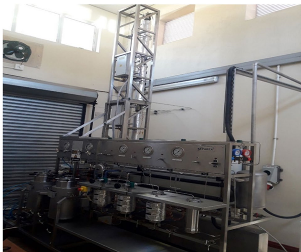
Fig. 1 Pilot plant set up for recovery of acetoin broth
