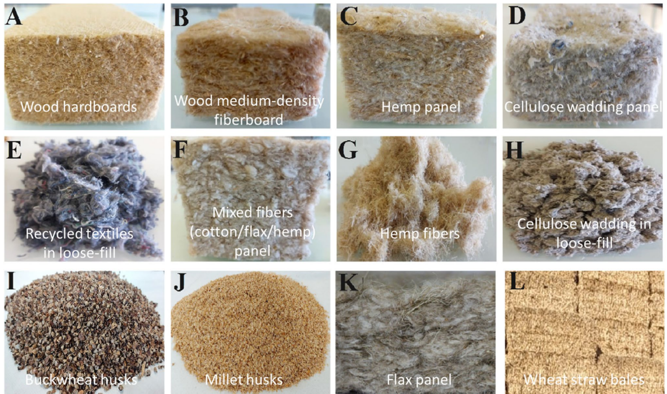
Fig. 3 Various biomass-based insulation materials and products (with permission and recreated using data published in [13])
