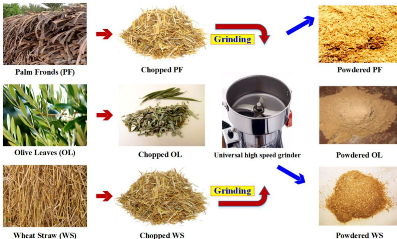
Fig. 1 Palm fronds (PF), oil leaves (OL), and wheat straw (WS) from the field, chopped and materials powders
