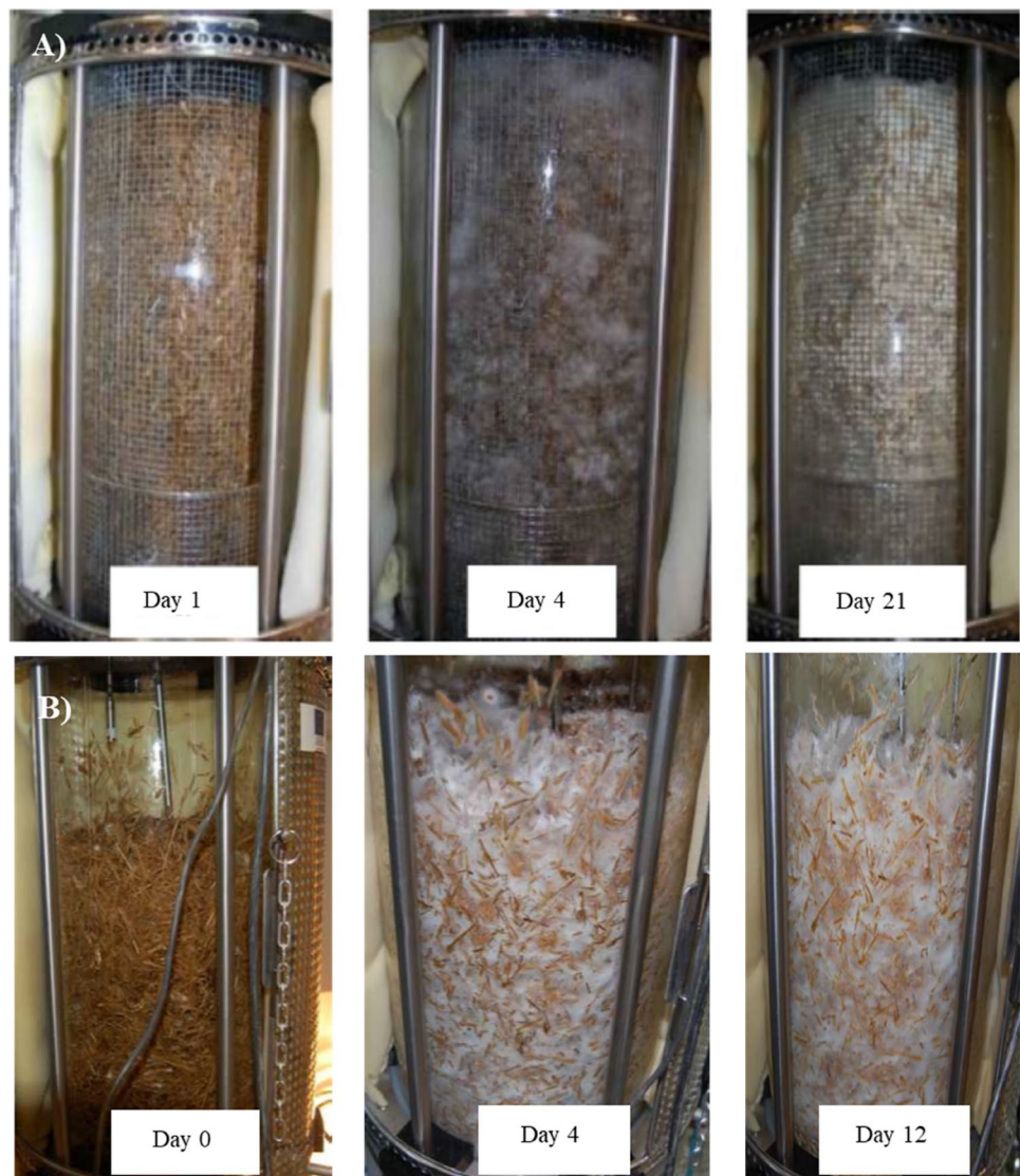
Fig. 2 Evolution of wheat straw during biological pretreatment with I. lacteus in the SSF reactor using the basket (A) and packed bed (B) configurations
