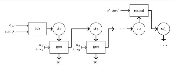
Fig. 1 A state machine representation of the NIST DRBG work flow
