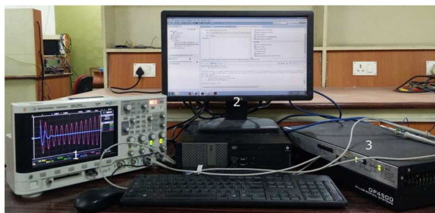
Real-time simulation process with OPAL-RT digital simulator
