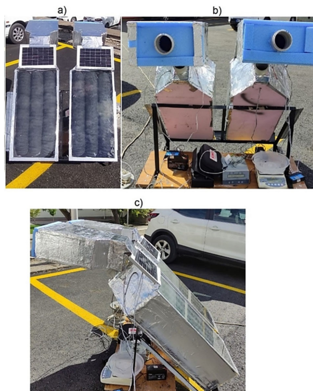
Fig. 5 (a) Front, (b) back, and (c) side views of the designed test rig
