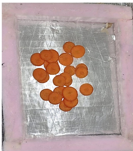
Fig. 4 Prepared carrot samples for drying and the utilized perforated tray
