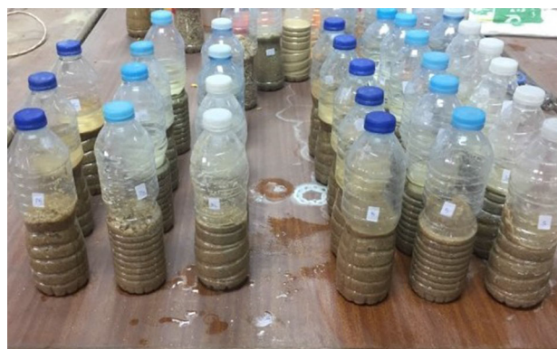
Fig. 1 Batch experiments on coarse silica sand and mix of zeolite nano-clay with coarse silica sand 1:30 using different concentrations of iron solutions
